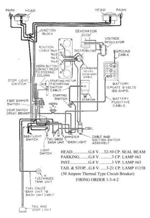
FIG. 16 -- WIRING DIAGRAM
